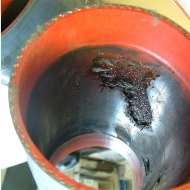
As visible in this photo, the critter often starts gnawing away at the inside surface of the hose over a period of time – without going through to the outside of the hose.
