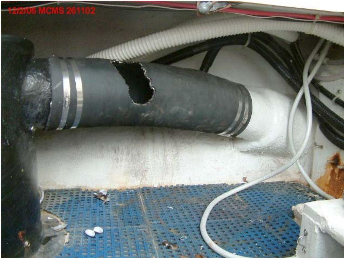
The hole in this hose is 6.5 by 2.5 inches and the bottom of the opening is even with the static waterline. Note small clamshells deposited under hose.
